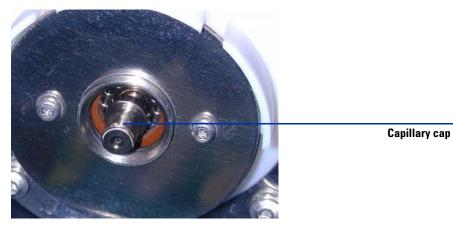
**Figure 12** Spray shield removed.
